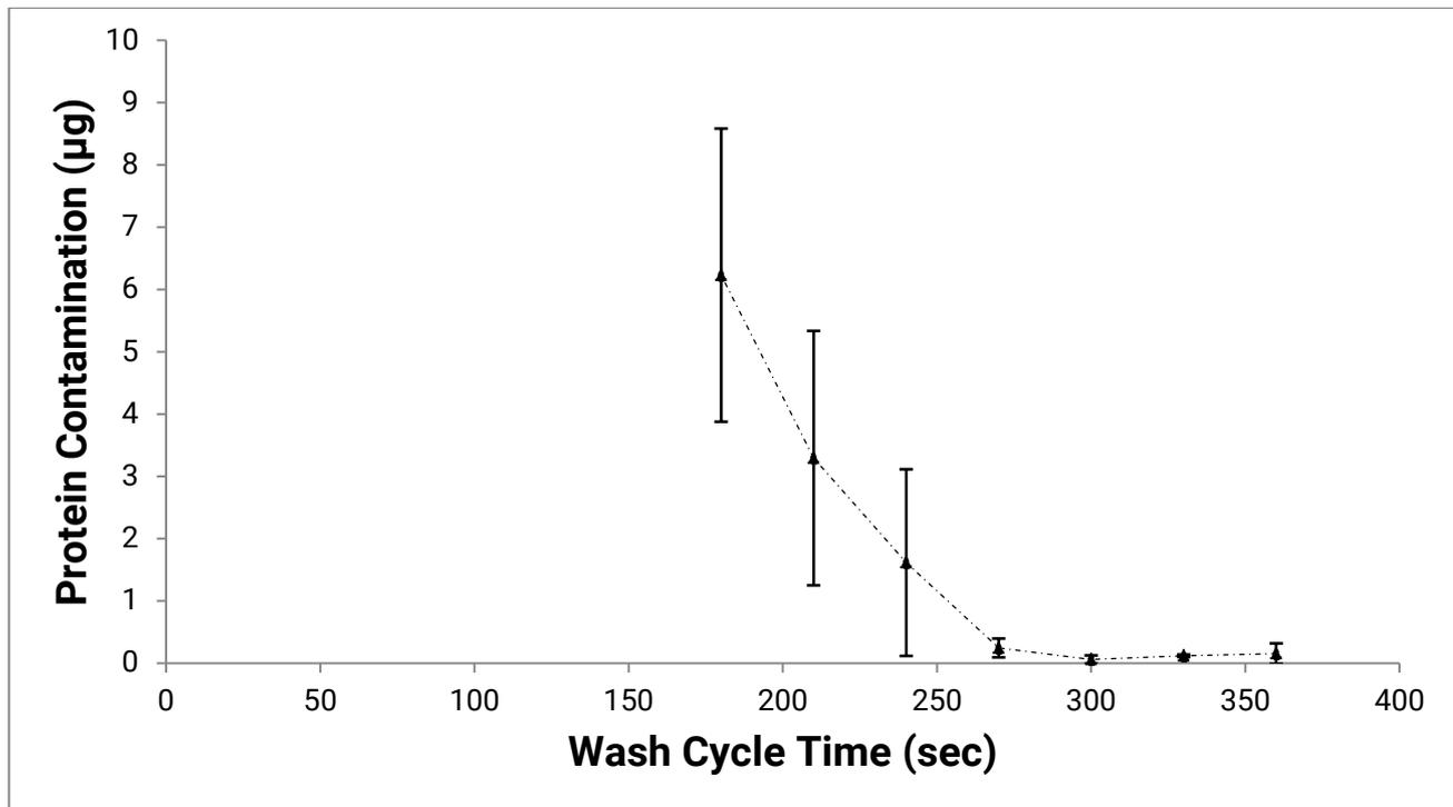
Figure 1: Process performance optimisation. Cleaning effectiveness with different wash cycle time. 7 different cycles were run: 180, 210, 240, 270, 300, 330 and 360 seconds. Each point is the average contamination of one tag (run with 4 replicates and  $n = 4$ ).
