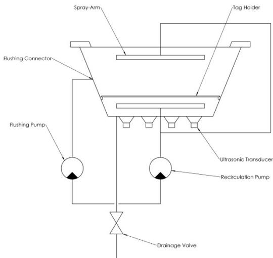
Schematic 1: Experimental washer-disinfector.
