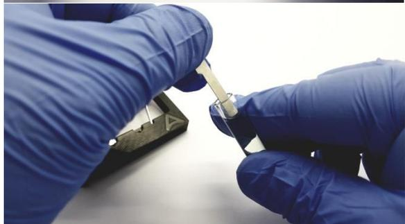
3. Holding the tag by the wider end or by the sides carefully insert the tag into the vial.
