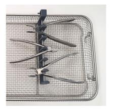
Keeps instruments at an angle, which means no residual water, and faster drying process. Keeps instruments open, which makes cleaning more effective.
